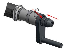
6. Nut runner with secured reaction arm and secured impact socket.
