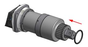
2. Attach the reaction arm to the toothed holder on the nut runner.
