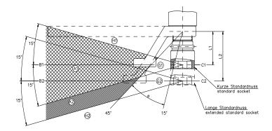
The location of the support surface depends on the respective length "L1 and L2" of the sockets. The ideal contact line is on the line "B1 - C1" or "B2 - C2". In this area, the force acting on the reaction arm is lowest.
