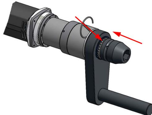
6. Nut runner with secured reaction arm and secured impact socket.
