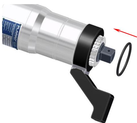
3. Plug a socket (nut) onto the square drive adapter at the nutsetter and secure it. Exclusively use sockets for use with power tools.
