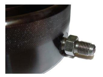
Screw the adaptor into the hydraulic cylinder.
