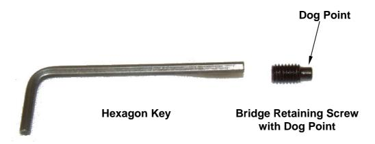
The screws remain in the Bridge but the Dog Point can be advanced into the groove machined in the recess, in the base of the Hydraulic Cylinder. A hexagon key is used to advance or withdraw the Bridge Retaining Screws working from the inside of the Bridge. It is not necessary to remove the screws for the Bridge and Cylinder to be separated. The screws need only be withdrawn into the Bridge wall by 2 to 3 mm to disengage the dog point from the groove.
