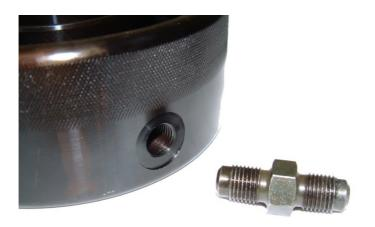
Check the internal and external threads are clean and free from damage
