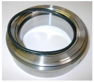
Lubricate the O Ring with grease
