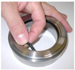
Fit the O Ring into the seal groove
