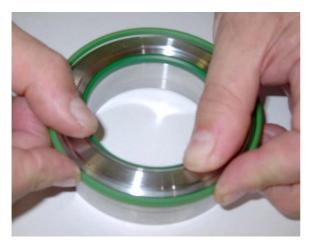
Insert the green plastic seal into the seal groove. Make sure the chamfer is at the top.
