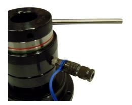
Using a tommy bar, gently wind the puller down the bolt, easing the piston into the cylinder. This should not require much force. The seals can be easily damaged if the piston is not aligned correctly with the cylinder.
