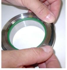
Stretch the O Ring until it snaps into the seal groove
