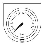
Release the pressure slowly. When the pressure has fallen to zero, fully open the oil pressure release valve on the pump.
