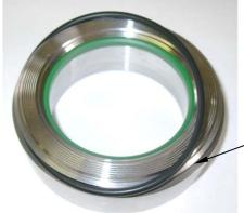
Lubricate the O Ring with grease.
