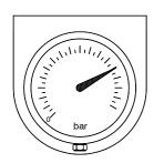
Apply the correct hydraulic pressure, observing the Health and Safety Instructions. The Piston will move out of the Cylinder as the bolt is stretched and the bolted joint is compressed.
