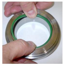
Work the seal into the groove using hand force only.
