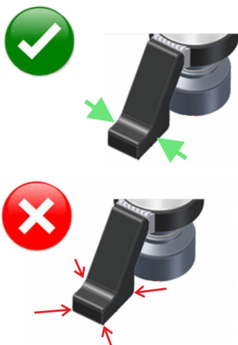
Fig. 14: Bracing the reaction arm correctly
