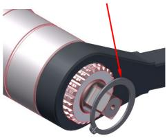
3. Put the accessory on the square drive on the battery gate valve wrench and secure it.
