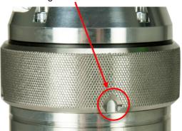
Pivot not locked ("free movement") This position is used only to perfectly position the battery gate valve wrench for the application
