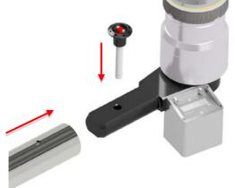
6. Illustration of secured reaction arm
