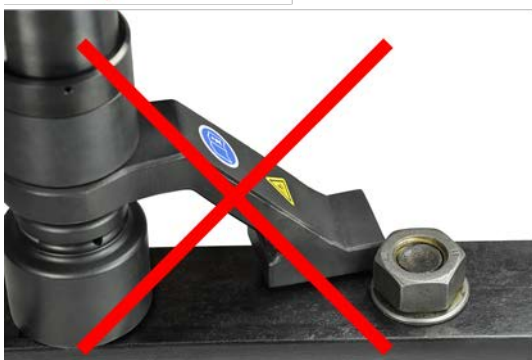
Incorrect support at the corner of the foot.
