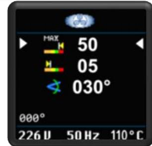
The tool tensions the bolt with the set snug torque level before turning the bolt further with the set tightening angle.
