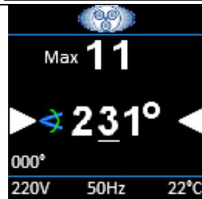
The tool tensions the bolt by applying  $M_{dmin}$  before turning the bolt further with the set tightening angle.
