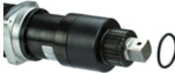
2. Attach the reaction arm to the toothed holder on the nut runner.
