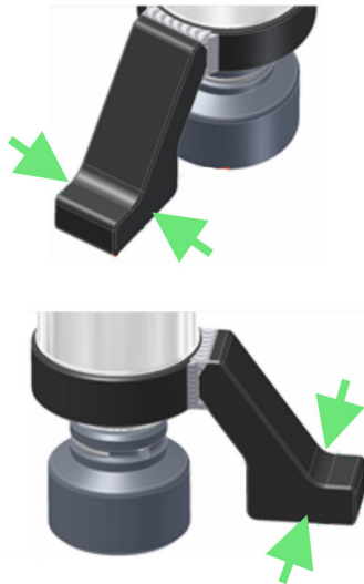
Fig. 18: Bracing the reaction arm correctly
