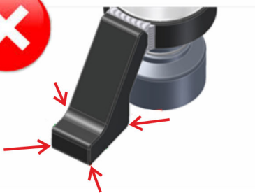
Fig. 19: Reaction arm braced incorrectly
