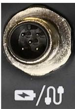
Fig. 14: Connection for remote control
