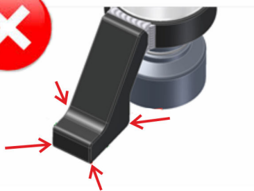
Fig. 19: Reaction arm braced incorrectly
