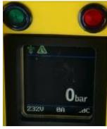
Reset the error message and reassume control of the power pack with a press of the “automatic” button.
