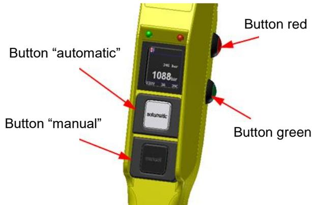
Navigate by using the button combination of red button and button “automatic” or “manual”.
